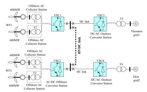
Fig. 4. Multi-terminal VSC-HVDC connection with DC-CBs.
