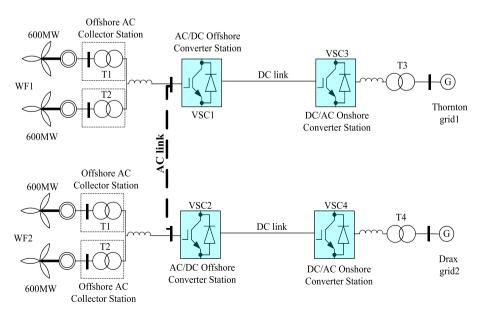
Fig. 5. point to point connection with auxiliary cable.
