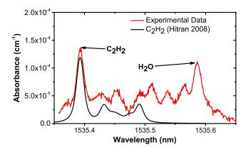
Fig. 5. Higher resolution spectrum acquired 3 mm above the burner in the 1.66 equivalence ratio flame. Also shown is a model spectrum of  $C_2H_2$  from the Hitran 2008 Database [24]. The p17e acetylene transition and  $H_2O$  transition are identified.
