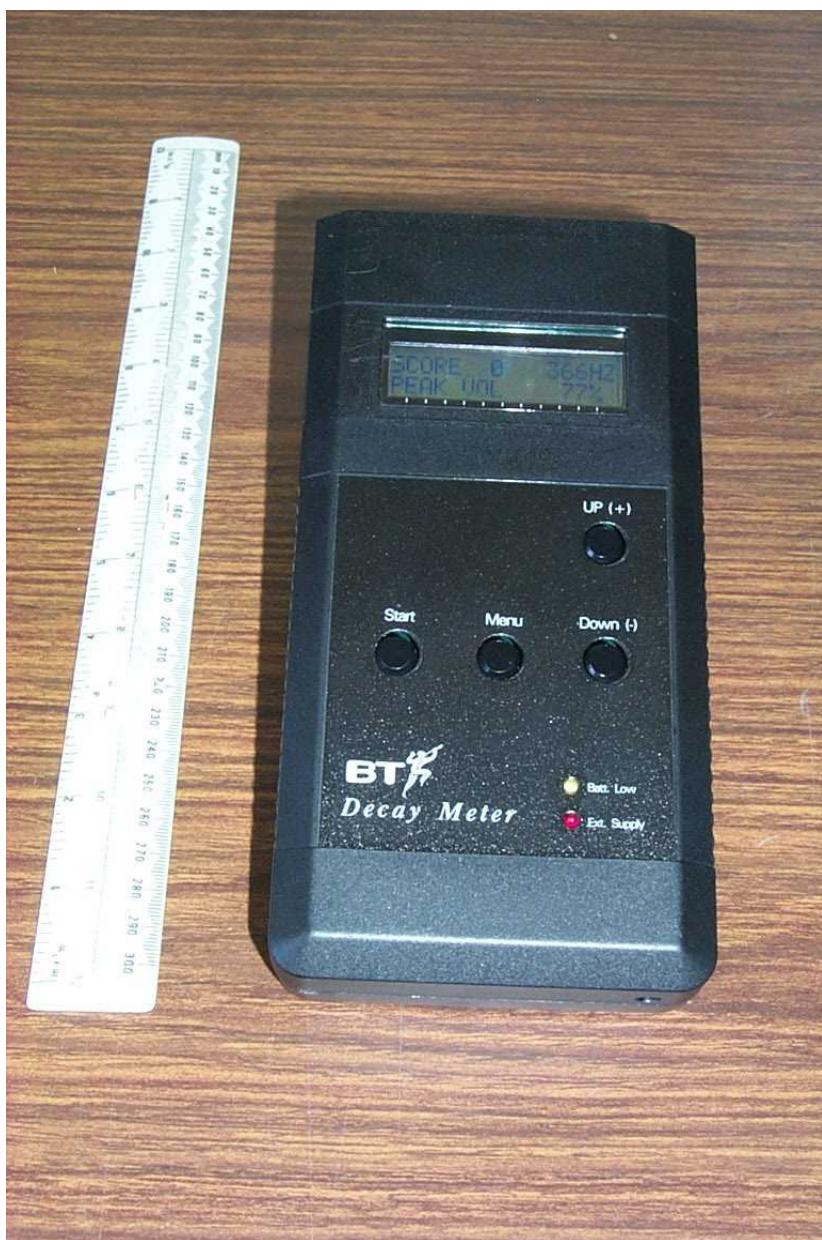
Figure 13 The pole decay meter.
