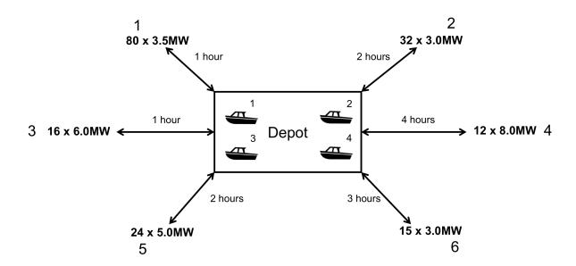
**Fig. 2.** Example central dispatch simulation, showing 6 offshore wind farms of varying installed capacity and model type, dependent on one onshore maintenance depot with 4 dispatchable maintenance teams.
