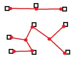
Figure 20: Radial HVDC systems
