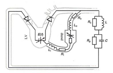
**Figure 10** Electric analog of LVAD model coupled with the circulation: LV, rotary blood pump in parallel and 4-element windkessel. From: Artificial Organs 2002; 26(12): 1032-1039 with permission from John Wiley and Sons.
