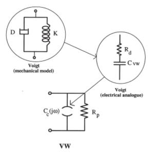
**Figure 6** Electric analogue of the viscoelastic Windkessel model (VW) derived from a Voigt cell. Reprinted from: Burattini R, Natalucci S. *Medical Engineering & Physics 1998; 20: 502-514* with permission from Elsevier.
