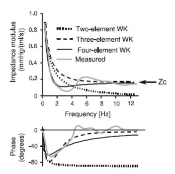
**Figure 5** Comparison of measured aortic input impedance with values predicted by the 2-element, 3-element and 4-element windkessel model. Reprinted from: Westerhof N, Lankhaar J-W, Westerhof BE. *Med Biol Eng Comput 2009; 47: 131-141*.
