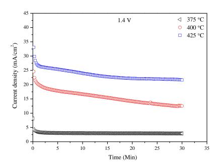
Fig. 5 Electrolytic cell performance stability at 1.4 V and 375-425  $^{\circ}$ C.
