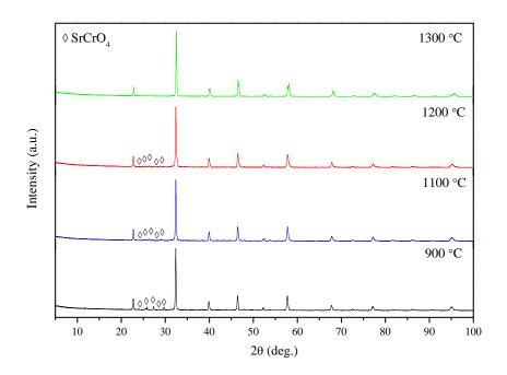
Fig. 1 XRD patterns of  $La_{0.75}Sr_{0.25}Cr_{0.5}Fe_{0.5}O_{3\text{-}\delta}$  at different firing conditions.
