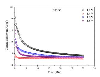
Fig. 8 Electrolytic cell performance stability at 375  $^{\circ}\text{C}$  and 1.2-1.8 V
