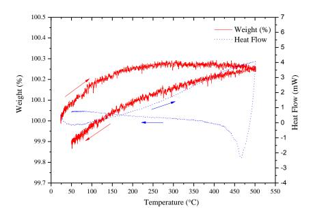
Fig. 4 TGA-DSC curves for perovskite based catalyst (LSCrF) in nitrogen, up to 500 °C
