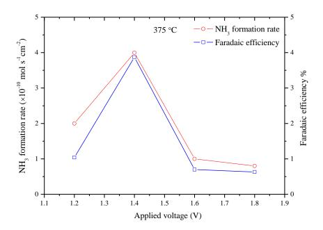
Fig. 9 Dependence of the rate of ammonia formation rate on the applied voltage at 375  $^{\circ}$ C
