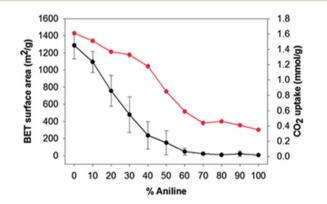
Fig. 7 Surface area (black) and CO<sub>2</sub> uptakes (red) of the anilinebenzene HXL materials depending on the feed ratio. Error bars calculated from measurements of three nominally identical networks at each % aniline. Reprinted from *Polym. Chem.*, 2012, **3**, 2034–2038. Copyright (2012) Royal Society of Chemistry.
