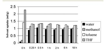
Fig. 4 Solvent uptake data of resins isolated at various times during the hypercrosslinking of gel-type VBC-DVB (98:2) precursor resin. Reprinted from *Macromolecules*, 2006, **39**, 627–632. Copyright (2006) American Chemical Society.
