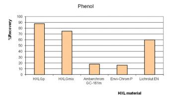
Fig. 5 Recovery values when 100 mL of a standard solution spiked with phenol, at a constant amount injected of 0.2  $\mu$ g, was percolated through a precolumn packed with HXL materials in SPE-LC-UV-Vis.
