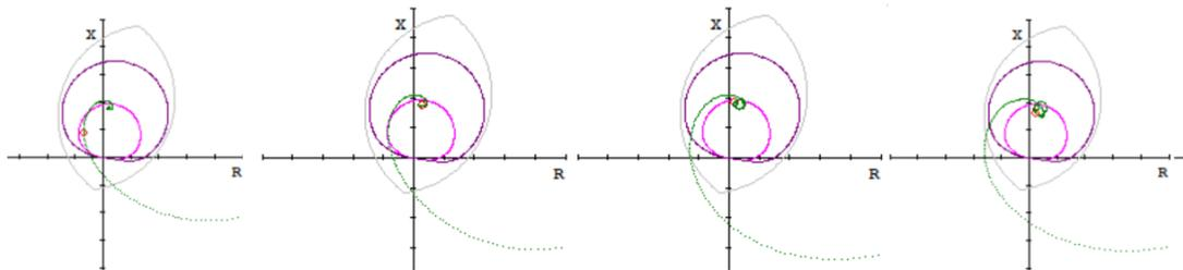
Fig. 7. Impedance loci as measured by the relay (from left to right: 1ms, 5ms, 10ms and 15ms converter initial delay)
