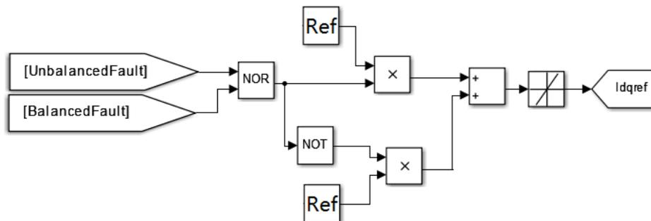
Fig. 3. Fault response logic (Ref: the reference value for the converter's inner control loop)
