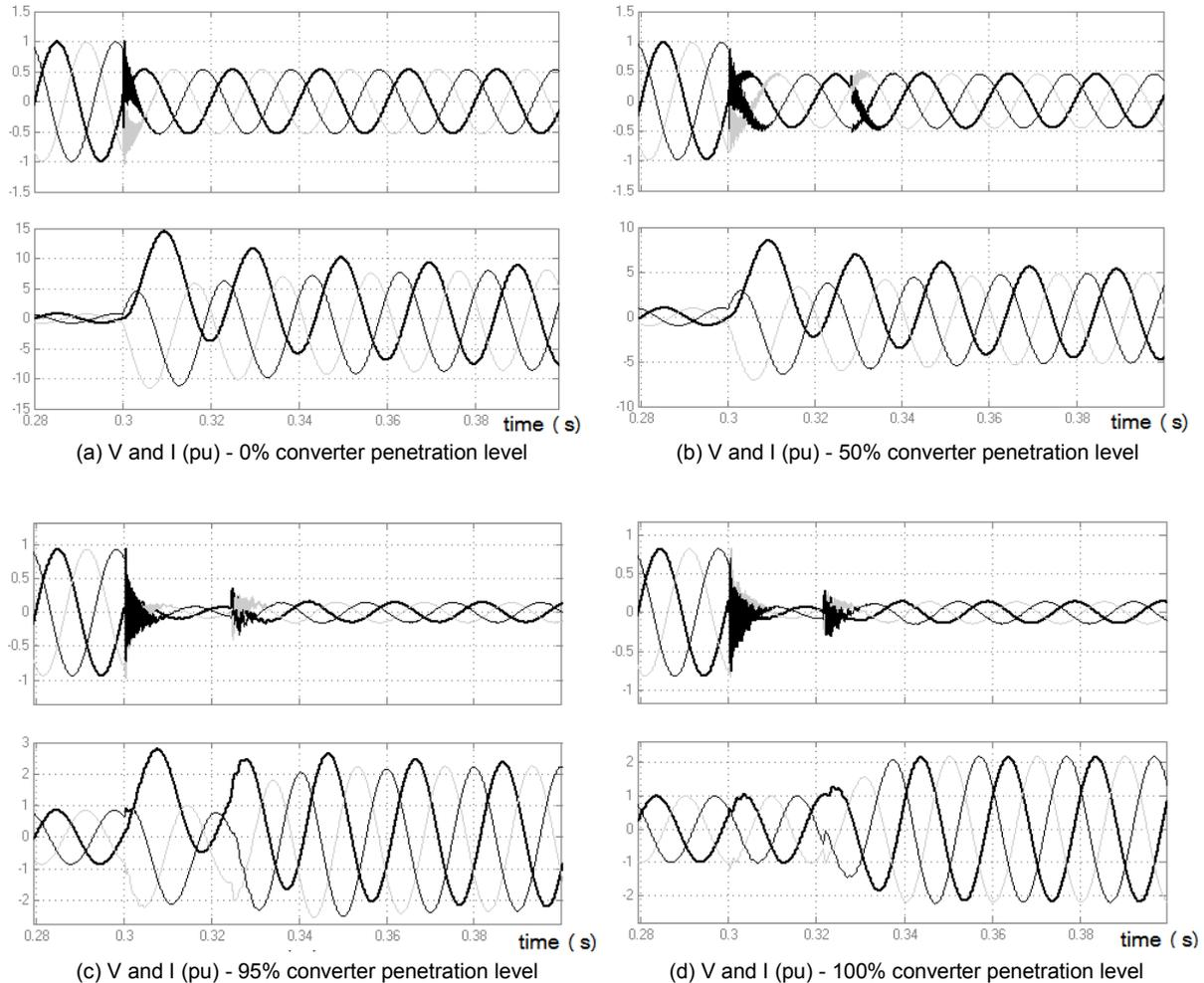
Fig. 5. Voltage (top traces) and current (bottom traces) (in pu) as measured at the sending end bus
