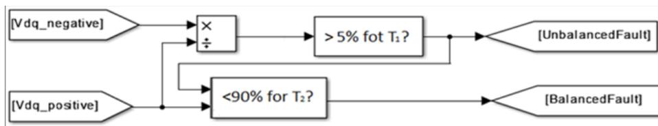
Fig. 2. Fault detection logic ( $T_1$ : required time for balanced fault detection;  $T_2$ : required time for unbalanced fault detection)
