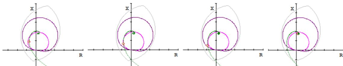
Fig. 8 Impedance loci for varying ramp rates (from left to right, 0.0035, 0.00245, 0.00175, 0.00112 pu/ms)
