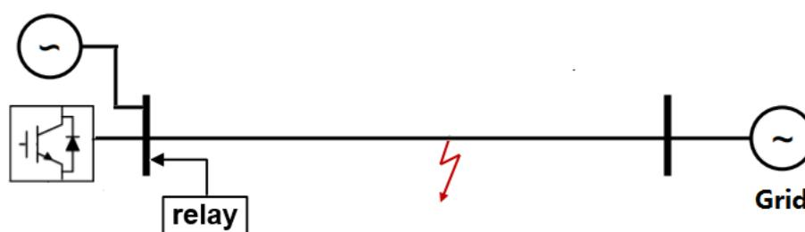
Fig. 4. Model of a transmission line supplied by a combination of synchronous/converter-interfaced sources.
