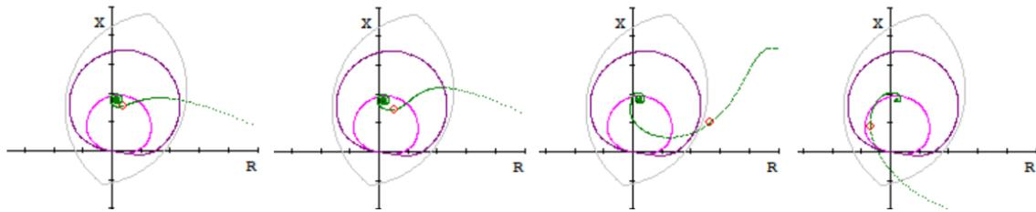
Fig. 6. Impedance loci as measured by the relay (from left to right: 0%, 50%, 95%, 100% penetration levels)
