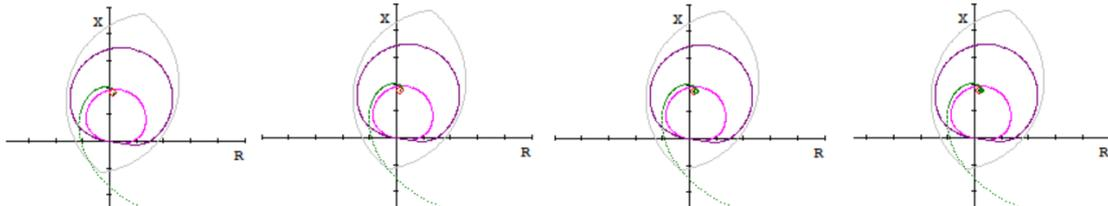
Fig. 9 .impedance loci for varying converter fault current levels (left to right, 1.1pu 1.4pu 1.8pu 2.2pu fault current)
