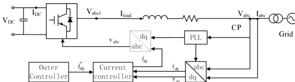
Fig. 1. Overall layout of the VSC system
