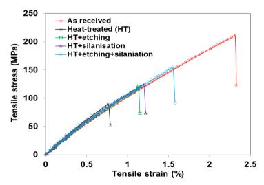
Fig 4 Typical tensile stress-strain curve obtained from CSM-epoxy composites with glass fibres received different treatments
