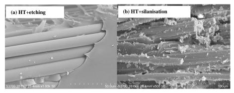
Figure 6 SEM photo of fractured area obtained from tested samples consisting of the CSM conditioned with (a) heat treatment at 500°C followed by HF etching and (b) the same heat treatment followed by APS silanisation
