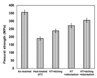
Figure 7 Flexural strength of CSM-epoxy composites with glass fibres received different treatments
