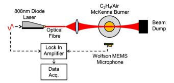
Fig. 1 Experimental set-up for photoacoustic soot measurement
