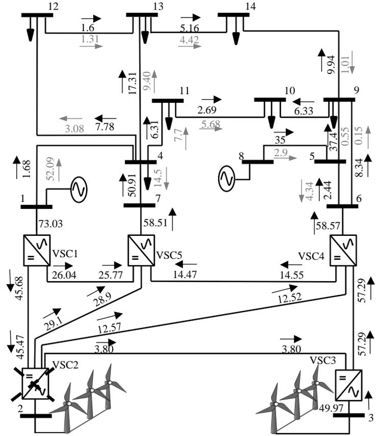
Figure 6: Modified IEEE14 network with five-terminal MTDC system
