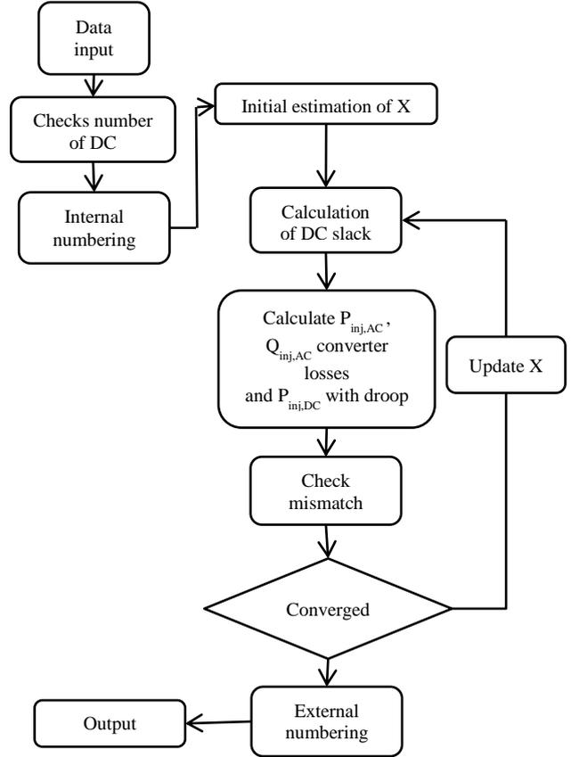
Figure 5: Flow chart for the combinational power flow
