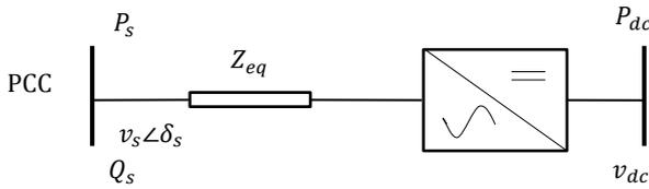
Figure 4: Control mode representation of the VSC station
