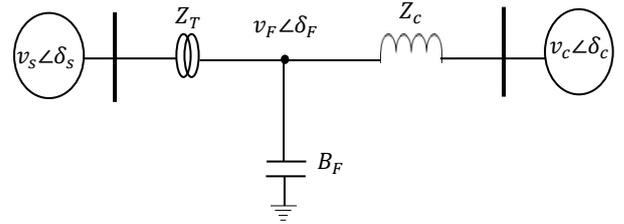
Figure 1: VSC station representation for power flow study
