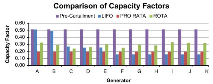
Fig. 3. Graph showing the changes in CFs for different PoA on Wind Generators.
