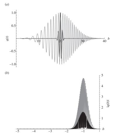
**Figure 1.** (a) A gated continuous sine wave with frequency  $f=1\,\text{MHz}$  modulated by a Gaussian envelope with parameters  $\sigma=1\,\mu\text{s}$ ,  $t_1=20\,\mu\text{s}$  (in black) and a Gaussian-modulated linear chirp with parameters  $\sigma=8\,\mu\text{s}$ ,  $t_1=20\,\mu\text{s}$ ,  $m=0.22\,\text{MHz}$  and  $f_1=0.1\,\text{MHz}$  (in grey). Their respective Fourier transforms (power spectra) are shown in (b).
