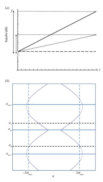
**Figure 4.** (a) Schematic demonstrating the increase in bandwidth with the increase of chirp rate m. The long-dashed line is representative of a single frequency pulse and its bandwidth is a delta function at that frequency. The dotted and solid lines represent linear chirps with increasing gradients which result in increased bandwidths. (b) Schematic demonstrating the change in  $\sigma_a$  in the fractional Fourier domain. (Online version in colour.)
