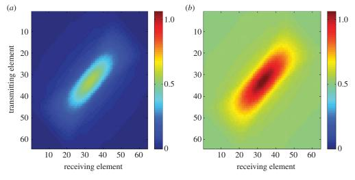
**Figure 3.** Sum of the scattering matrices as generated by the Born approximation arising from (a) gated continuous wave excitation and (b) linear chirp insonification. (Online version in colour.)
