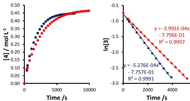
**Figure 4.** Kinetic data for the RCM of 3 (0.5 mol L<sup>-1</sup>, toluene-*d*<sub>8</sub>, 288 K with 250 ppm pre-catalyst), monitored by <sup>1</sup>H NMR spectroscopy: (a) concentration/time profiles; (b) first order treatment of kinetic data; SIPr in blue, SIPr<sup>OMe</sup> in red.
