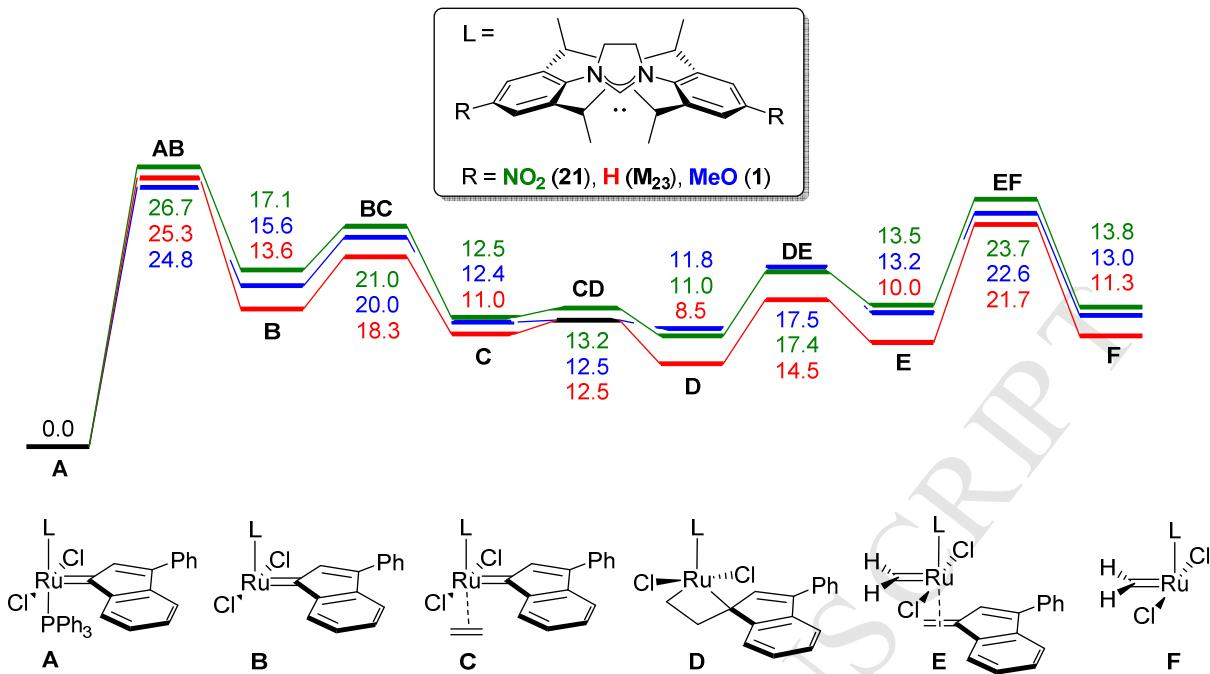
**Figure 5.** PESs for the metathesis of ethene by **1**, **M<sub>23</sub>** and **21**.
