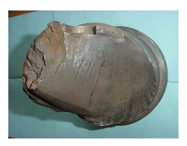
Figure 1 View of fractured shaft looking from coupling end towards generator.
