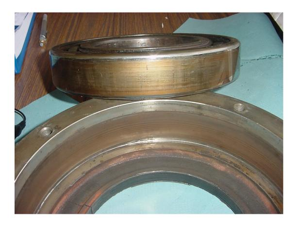
Figure 2 View of bearing and housing showing circumferential wear and marking.
