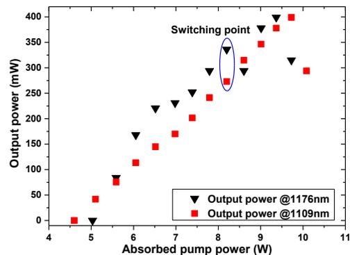
Fig. 4. Power transfer of Raman lasers resulting from the 379cm<sup>-1</sup> transition (in red) and the 893cm<sup>-1</sup> transition (in black).
