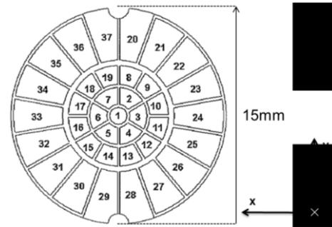
Fig. 2. Actuator designation of deformable mirror.
