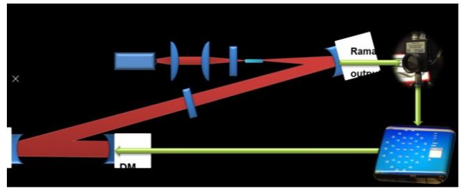
Fig. 1. Diagram of the Nd:YVO<sub>4</sub> self-Raman laser incorporating the AO feedback loop.
