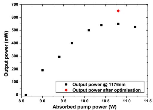
Fig. 3. Power transfer of the  $\lambda = 1176$ nm output before optimization including the post-optimisation result.
