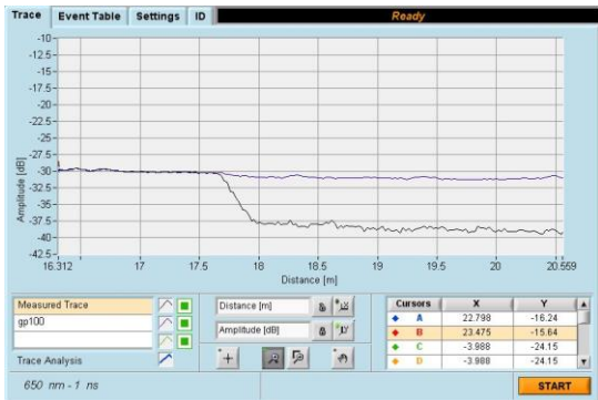
Figure 7: High resolution OTDR trace of the attenuation introduced at 17.6m by moistening a section approximately 30 cm long using a hand-held water spray.
