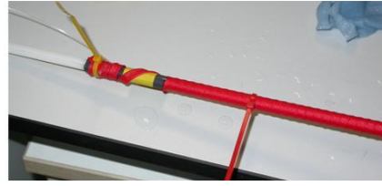
Figure 6: Photograph of the laboratory bench mock up sensor. The red wrap is a porous tape and the sensor is approximately 8mm in diameter
