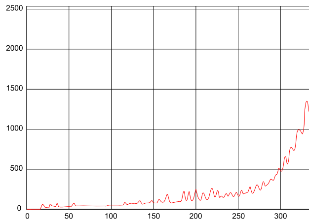
Fig. 14. Floodwater (t) versus time (s) for 0.1 \text{ m}^2 cardeck downflooding opening area each. (Colors are visible in the online version of the article; http://dx.doi.org/10.3233/ISP-130109 .)
