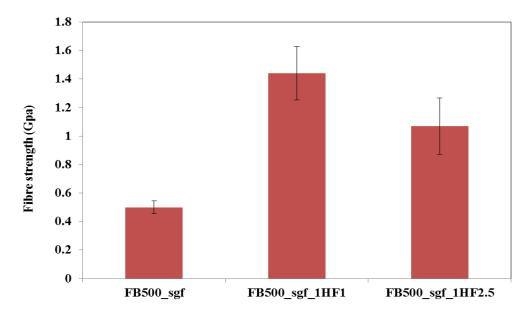
Figure 4. Tensile strength of fludised bed-recycled glass fibre after 1wt% HF treatment
