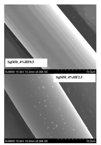
Figure 3. SEM photos of glass fibre treated by 4 wt% HF solution
