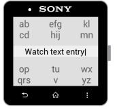
**Figure 1:** Prototype smartwatch text entry on Sony SmartWatch 2
