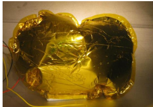
Figure 2: Inflated cell in vacuum chamber
