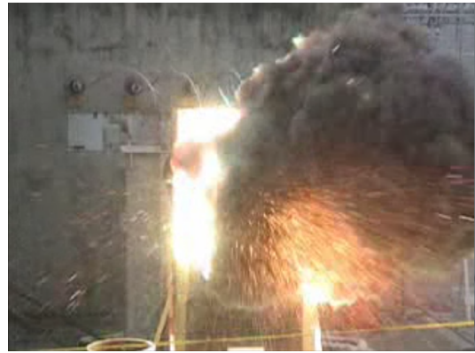
(b) 480 V arc flash experiment [Sho11]
