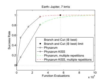
Figure 5: Success rate: Physarum, Physarum KISS and Branch & Cut. Earth to Jupiter transfer EJ7,  $v_{\infty,L} = 7km/s$ ,  $\alpha = 1.5\pi$ .
