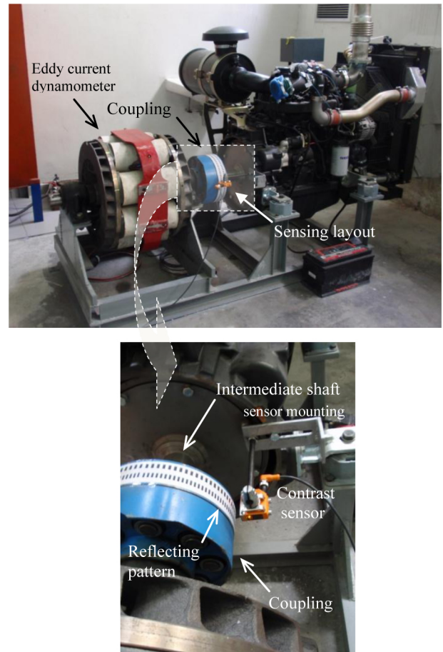
Figure 8. The developed system integrated on the IVECO N45 MST engine
