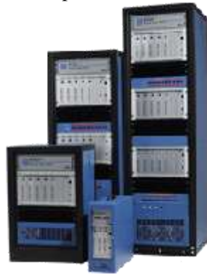
Figure 5 The Real-Time Digital Simulator – RTDS [12].
