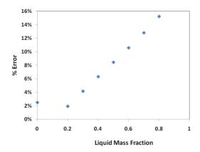
Fig. 6 CFD – Experimental Error (The data has been fitted to allow the difference to be calculated at corresponding liquid mass fractions)
