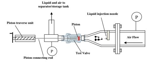
Figure 3 Schematic of valve two phase test facility
