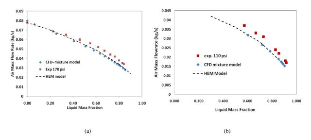
Fig. 5 Air mass flow predictions for CFD and HEM models against experimental data
