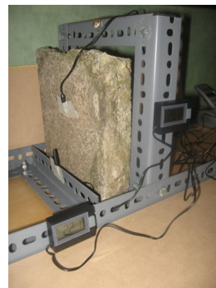
Figure 4 - Thermometers T2 and T3 in place
