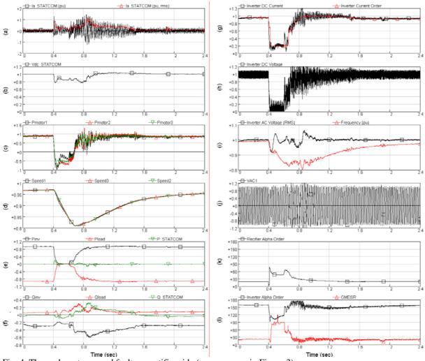
Fig. 4 Three-phase to ground fault on rectifier side (same axes as in Figure 3)
