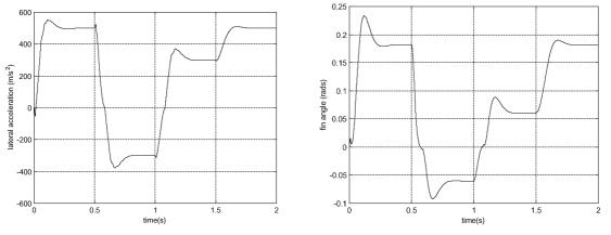
Fig. 7. Step responses with nominal plant and velocity-based gain-scheduled controller.
