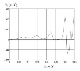
Fig. 1. Response of the closed-loop system to an acceleration step demand of  $100\,m/s^2$  with the classical gain-scheduled controller.
