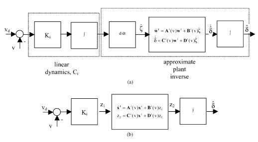
Fig. 2. Alternative formulations of inner-loop controller.
