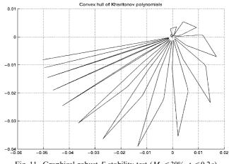
Fig. 11. Graphical robust  $\Gamma$ -stability test ( $M_p \leq 30\%$ ,  $t_s \leq 0.2$  s).
