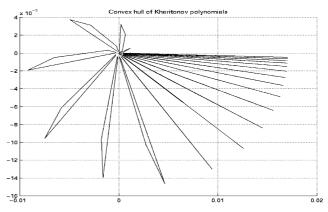
Fig. 10. Graphical robust  $\Gamma$ -stability test ( $t_s \leq 0.2$  s).
