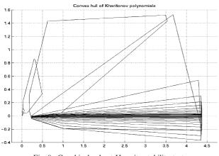
Fig. 8. Graphical robust Hurwitz stability test.
