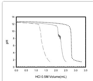
**Figure 2 pH curves from titration analysis.** Curves from titration by 0.5 M HCl of (⋯):1.4 mL of 1.0 M NaOH, (—): Native starch treated with 1.4 mL 1.0 M NaOH, (—): Native starch and decanoic acid mixture treated with 1.4 mL 1.0 M NaOH.
