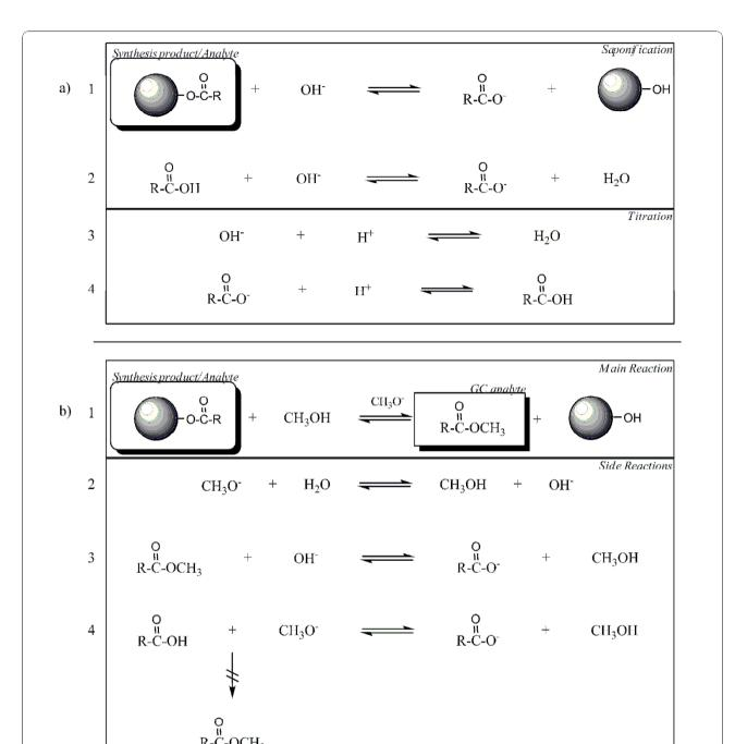
Figure 1 Reactions and side-reactions of starch ester analyses. a) Titration Analysis: 1 Hydrolysis of starch ester (circle denotes starch), 2 Saponification of acid, 3 Titration of residual hydroxide ions, 4 Titration of saponified acid, b) Transesterification/GC Analysis: 1 Methanolysis of starch ester and formation of methyl ester, 2 Hydrolysis of methoxide 3 Hydrolysis of methyl ester, 4 Deprotonation of acid to form acyl ion, no methyl ester synthesis.
