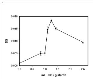
**Figure 5 Change in obtained DS for different initial concentrations of tapioca starch/water mixtures.** This shows the ratio of starch to water mixed prior to the gelatinisation stage. Water content of the starch, and water losses were negligible, but additional water is present during the enzyme reaction, because this is added as an aqueous solution (0.5 mL per g starch). Reaction time was 1 hr.
