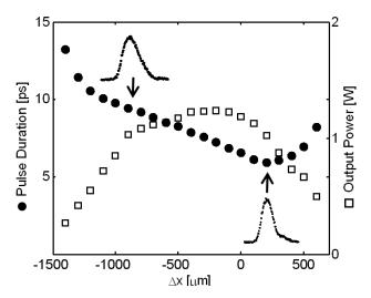
Fig. 4 Output pulse duration (filled circles) and Output power (open squares) changing the cavity length for the 2nd Stokes. (inset) Cross correlations of the output orange pulses for different cavity length detunings.
