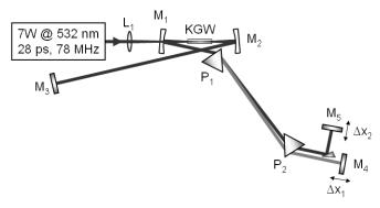
Fig. 1. Setup for the multi-cavity continuous-wave mode-locked Raman oscillator.
