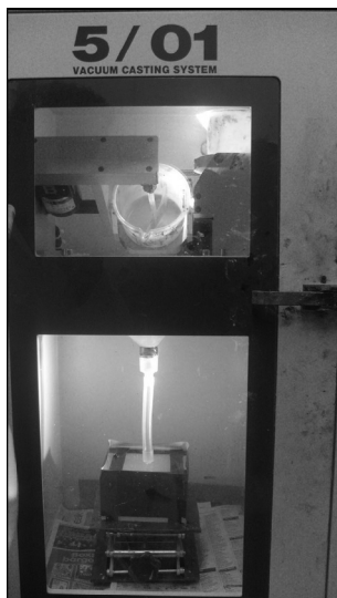
Fig 19: Vacuum casting Impeller
