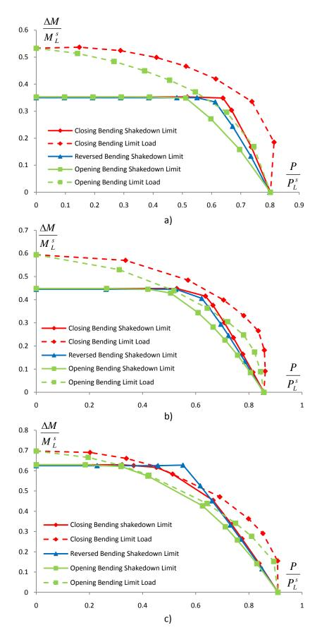
Figure 15 - Comparison of Closing and Opening Bending for fixed r/t=10 and a) R/r=2, b) R/r=3 and c) R/r=5
