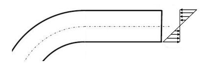
Figure 3 - Application of Pure Bending Moment Using the DLOAD Subroutine
