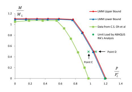
Figure 8 - Comparison of LMM with Data from C.S. Oh et al for R/r=2, r/t=10 Subject to Internal Pressure and Opening Bending
