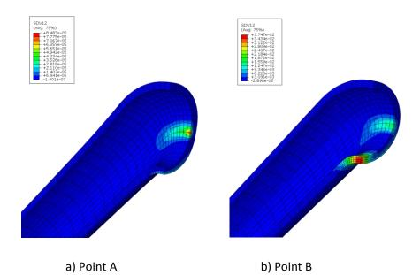
Figure 7 - Contour Plots of Plastic Strain to Show Failure Mechanisms of a) Alternating Plasticity at Point A and b) Ratcheting at Point B
