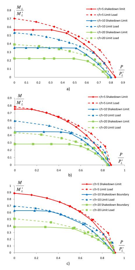
Figure 11 - Effect of changing r/t with a) R/r=2, b) R/r=3 and c) R/r=5, opening bending
