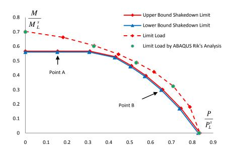
Figure 6 - Shakedown Limit and Limit Load curves for R/r = 2, r/t = 5, Internal Pressure and Opening Bending
