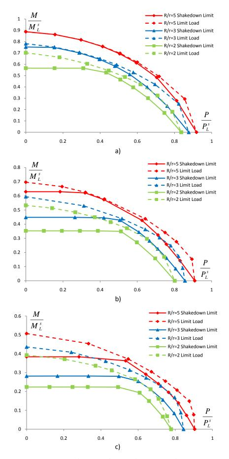
Figure 13 - Effect of Changing R/r with a) r/t=5, b) r/t=10 and c) r/t=20, opening bending
