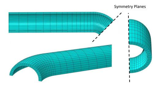
Figure 2 - Typical Meshed FEA Model
