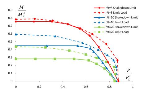
Figure 12 - Effect of changing r/t with fixed R/r=3, closing bending
