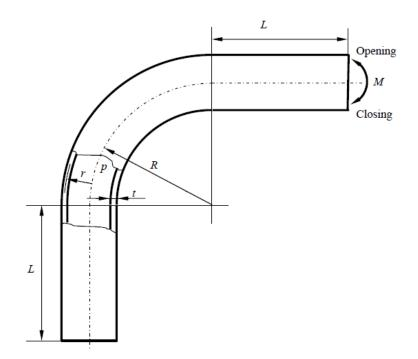
Figure 1 - Pipe Bend with Attached Straight Sections
