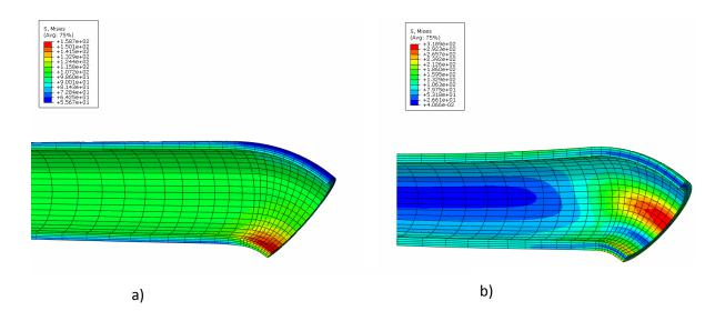
Figure 5 - Elastic solutions for a) Internal Pressure and b) Opening Bending
