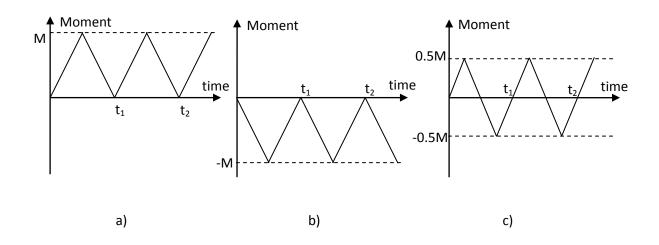
Figure 4 - Application of Cyclic Bending Moment During Shakedown Analysis for a) Opening Bending, b) Closing Bending and c) Reversed Bending
