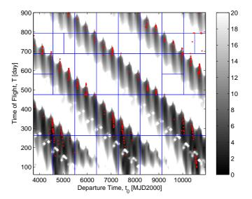
Figure 1: Characterization of the solution space for the Earth-Apophis transfer. The plot represents the areas in the solution space with low  $\Delta v$ , dark grey, and high  $\Delta v$ , light grey. The  $\Delta v$  is in km/s. The dots are all the solutions in the archive X.
