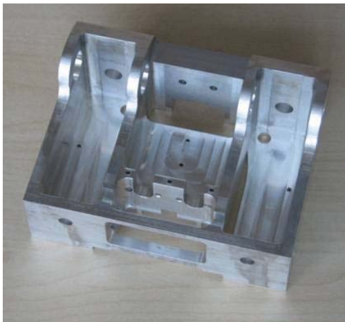
Fig. 5. Single aluminium unit that supports two actuators
