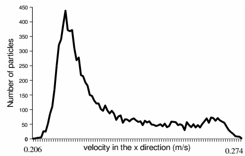
Figure 3: The horizontal component of the velocity of the particles as they enter the boundary area.
