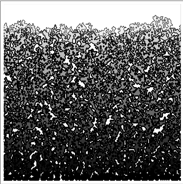
Figure 7: A Monte Carlo simulation of a compacted deposit ( 2.5 \times 10^6 mono-dispersed particles).
