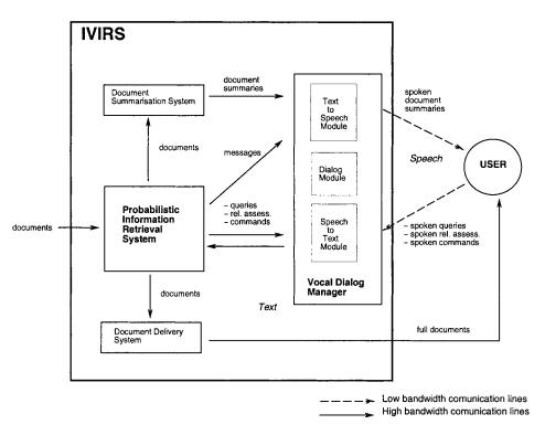
FIG. 1. Schematic view of the IVIRS prototype.
