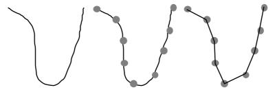
Figure 3 Approximation of a curve by 8-element polyline.
