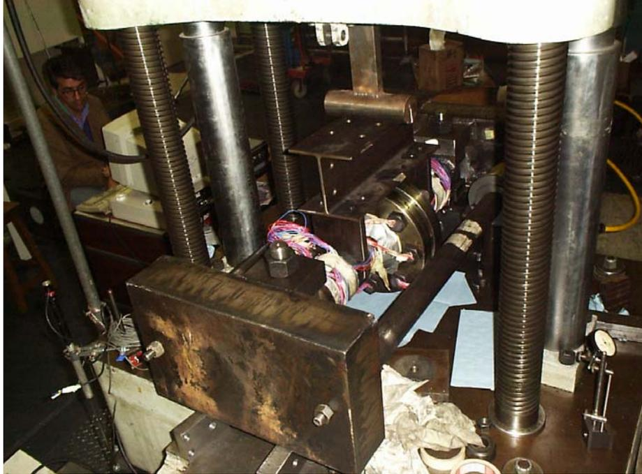
**Plate 1** Standard, gasketed joint under combined loading
