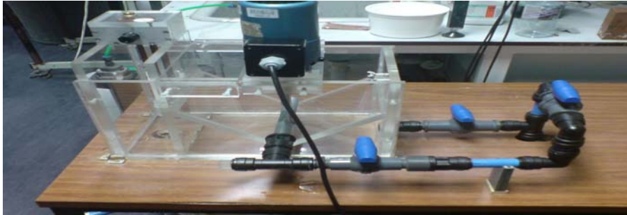
Figure (1) Erosion-corrosion test rig
