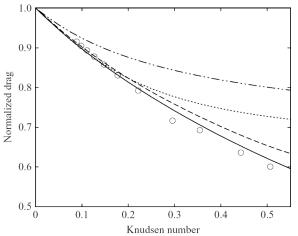
**Figure 2.** Flow around a sphere at various Kn, normalized drag force, comparing predictions using the near-wall constitutive scaling model of Lockerby and Reese (- -) with Basset's classical slip solution (- · · -), Cercignani's 2<sup>nd</sup>-order slip solution (· · ·), BGK kinetic theory results ( $\circ$ ), and experimental data (-). (Reprinted with permission from DA Lockerby, JM Reese (2008) On the modelling of isothermal gas flows at the microscale. *J. Fluid Mech.*, 604:235-261.)
