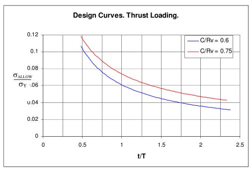
Figure 6. Design Curves for Thrust Loading.
