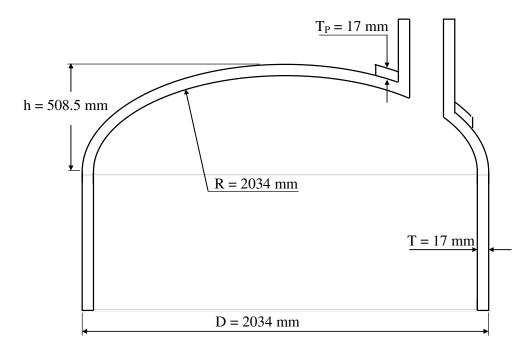
FIGURE A1. Vessel Dimensions.
