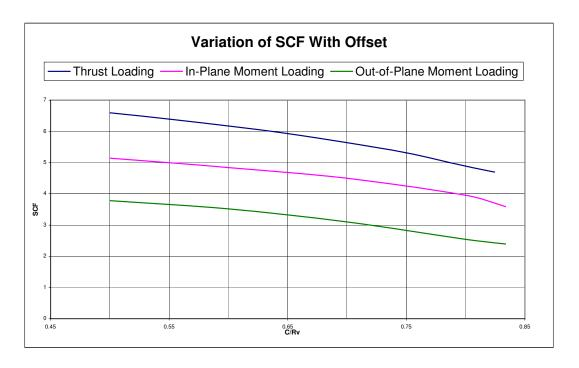
Figure 9. Stress Concentration Factor Variation With Nozzle Offset.
