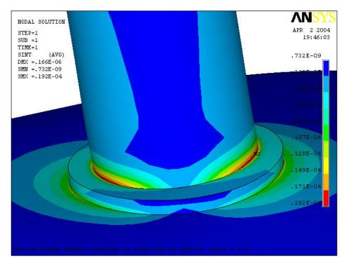
Figure 5. Stress Intensity Contour Plot. 8" Sch 40.  $D_P/d=1.3$ .  $C/R_V=0.6$ .
