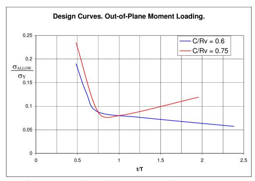
Figure 8. Design Curves for Out-of-Plane Moment Loading.
