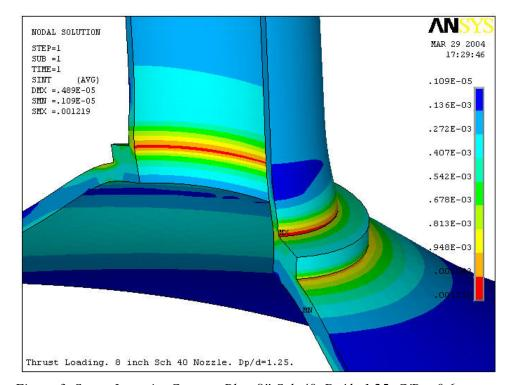
Figure 3. Stress Intensity Contour Plot. 8" Sch 40.  $D_P/d=1.25$ .  $C/R_V=0.6$ .
