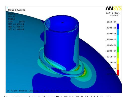
Figure 4. Stress Intensity Contour Plot. 8" Sch 40.  $D_P/d=1.3$ .  $C/R_V=0.6$ . For out-of-plane moment loading, curves for the two offsets converged on the same value of SCF. Convergence of the two curves occurred at different values of  $D_P/d$  for each nozzle. The value of  $D_P/d$  for convergence to occur was linked to both t/T and t/T and
