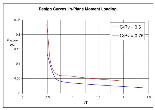
Figure 7. Design Curves for In-Plane Moment Loading.
