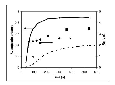
Figure 2. Comparison of spectrophotometric (left axis) and particle size (right axis) data for two different supersaturation values. Samples were prepared by injecting 100 µl of 50 mg/ml aqueous valine solution into valine saturated isopropanol: 15 ml (solid line, diamonds), 10 ml (dotted line, squares).
