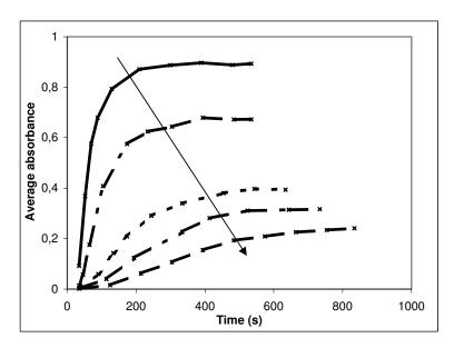
Figure 1. Spectrophotometric data on valine crystallisation kinetics. Samples were prepared by injecting 100 µl of 50 mg/ml aqueous valine solution into various volumes of valine saturated isopropanol ranging from 10 to 15 ml (arrow indicates increasing isopropanol volume).
