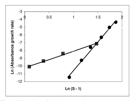
Figure 3. Dependence of absorbance growth rate on supersaturation. Samples were prepared by injecting 100  $\mu$ l of 50 mg/ml aqueous valine solution into various volumes of valine saturated isopropanol (circles). Results for subsequently diluted samples are also shown (squares).
