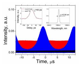
Fig. 2. Typical Nd:YVO $_4$  laser output traces under different external pump powers applied to the SA (0 W – black line, 0.74 W – red line, 0.89 W – blue line) and fixed pump power of the laser crystal (6 W). Inset: left – intensity autocorrelation trace of the  $\it cw$  ML pulse, right – corresponding optical spectrum.
