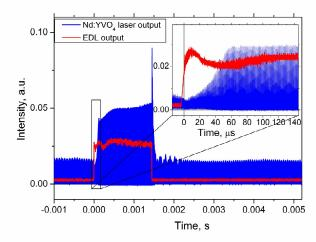
Fig. 4. Typical temporal response of rapid state-switching of the  $Nd:YVO_4$  laser (blue). The applied EDL control pulse is also shown (red).
