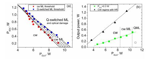
Fig. 3. (a) Map of laser oscillation state dependence on DLA and EDL power. The shaded region corresponds to the *cw* ML regime. (b) Nd:YVO<sub>4</sub> laser output power as a function of DLA power at constant EDL power = 0.3 W. Open symbol corresponds to optical damage of the SA. (The power transfer characteristic of the Nd:YVO<sub>4</sub> laser with the SA replaced by an HR mirror is shown for comparison.)
