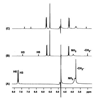
**Fig. 4** <sup>1</sup>H NMR spectra showing (A) di-Pt and (B) di-Pt with added Q[7] at R = 1 and (C) di-Pt with added Q[8] at R = 1 in D<sub>2</sub>O at 25 °C.
