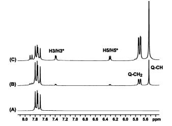
**Fig.** 7 <sup>1</sup>H NMR spectra showing (A) the hydrolysed form of tri-Pt and with added Q[7] at (B) R = 7.5 and (C) R = 2.5.
