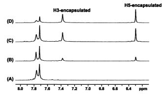
Fig. 5 <sup>1</sup>H NMR spectra showing (A) the hydrolysed form of di-Pt and with added Q[7] (B) 30 min, (C) 8 hours and (D) 15 hours after mixing.
