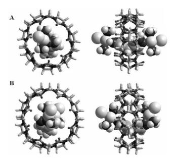
**Fig. 8** Molecular model of di-Pt encapsulated in (A) Q[7] and (B) Q[8] generated using HyperChem. The platinum complex was inserted into the cucurbituril in a variety of different starting positions. Energy minimisation of the encapsulated-di-Pt was then carried out to convergence.
