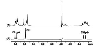
**Fig. 2** <sup>1</sup>H NMR spectra showing (A) Q[7] and (B) Q[7] with added cisplatin at R = 1 in D<sub>2</sub>O at 25 °C.
